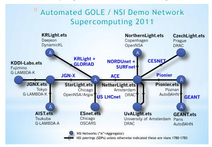
nodes that use the NSI protocol to re-configure the GOLE switches along a selected path to establish a dedicated VLAN between the two end points. This VLAN can be reserved in advance for a specified time, and is provisioned with dedicated capacity and
