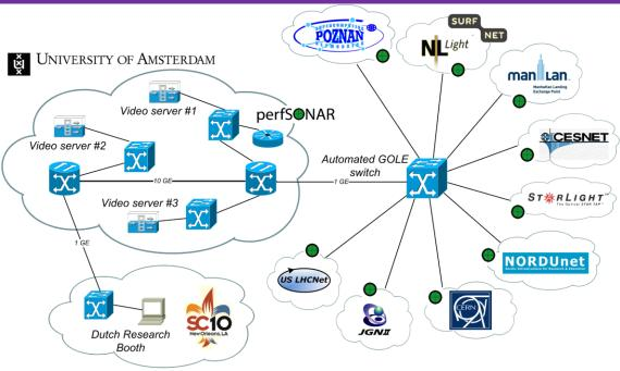
**SC10 demo setup.** This demonstration shows the dynamic setup of lightpaths through the Automated-GOLE infrastructure. Each domain has a PerfSONAR instance deployed that signals when domains are connected and is visualized in a pinger-matrix. Additionally, dynamic lightpath setup is demonstrated by connecting to different streamers showing distinct videos.
