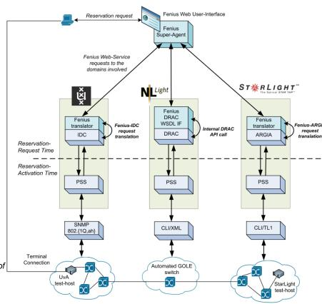
An example scenario of the interoperating Fenius – and NRPS systems. In this scenario a request for a path is made from an endpoint in the UvA network to an endpoint in StarLight traversing through the Automated GOLE infrastructure.
