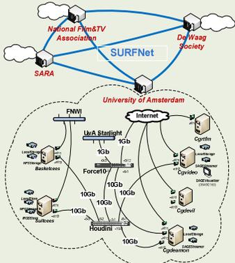
The goal of the **digital media delivery on demand** use case is to retrieve media material from the infrastructure, and request quality guaranteed connections to deliver the data to qualified nodes for further processing, such as playback or visualization.
